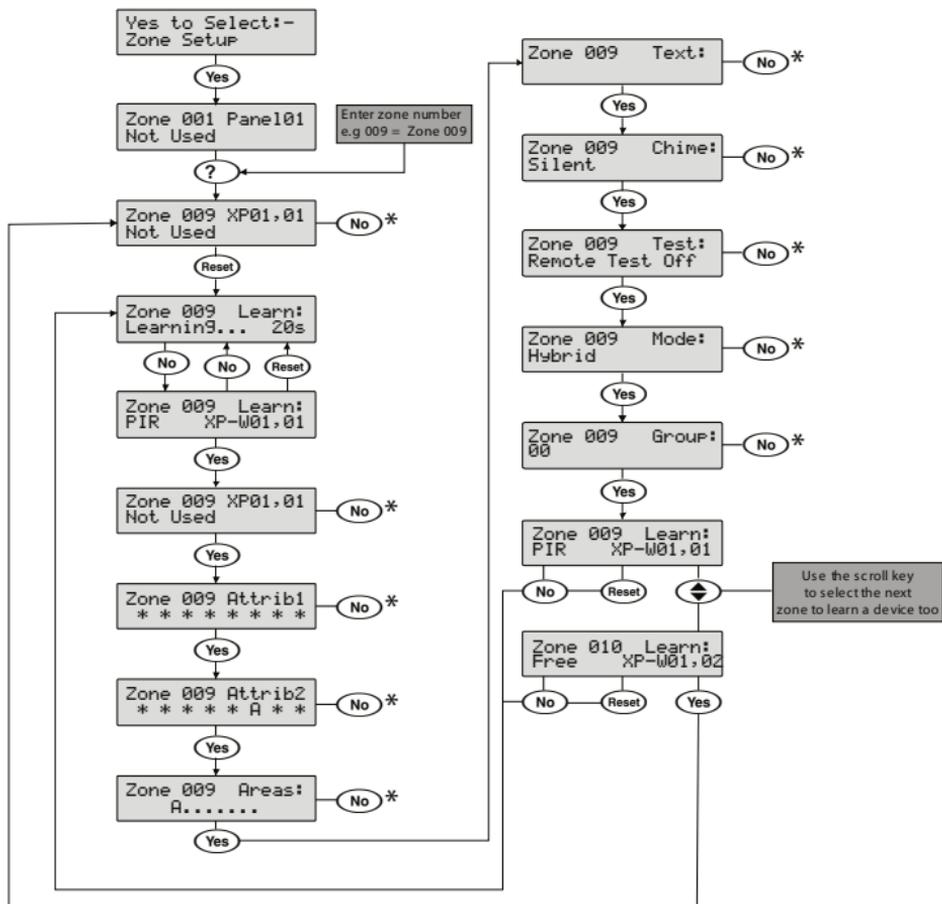
\* Please refer to INS176 "Zone Setup" for details when using the **No** key to change these settings
