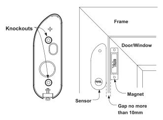
Note:The Door/Window Contact and magnet can be changed round as long as there is no more than a 10mm gap.
