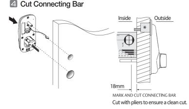
Place the electronic keypad in the hole on the outside of the door.
