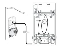
Feed the cable through the slot and then, being careful not to overlap it, zig-zag any excess cable behind the battery pack.
