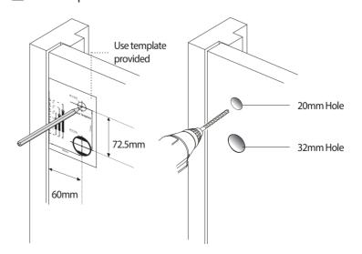
At the height you want your lock, use a pencil to mark a spot exactly 60mm from the edge of the door. At that spot, drill a 32mm diameter hole through the door.
