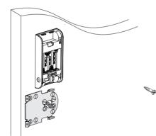
Fix screw to completely secure battery pack.
