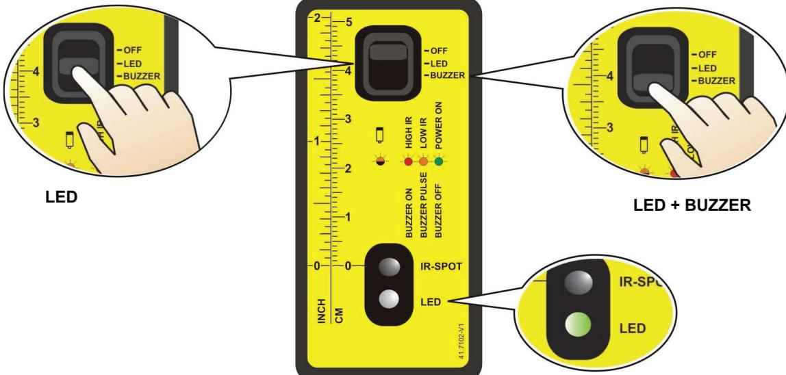
**UK** When switching ON, the GREEN LED lights up. You can choose between two positions: LED-signal only or both LED-signal and BUZZER tone. Note that the SPOTFINDER deactivates itself after 45 seconds without detection of IR-light. To reactivate, switch OFF and ON again.
